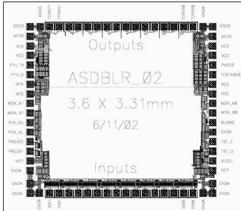
Figure 5: Bonding diagram of the ASDBLR chip in the FBGA packaging.
