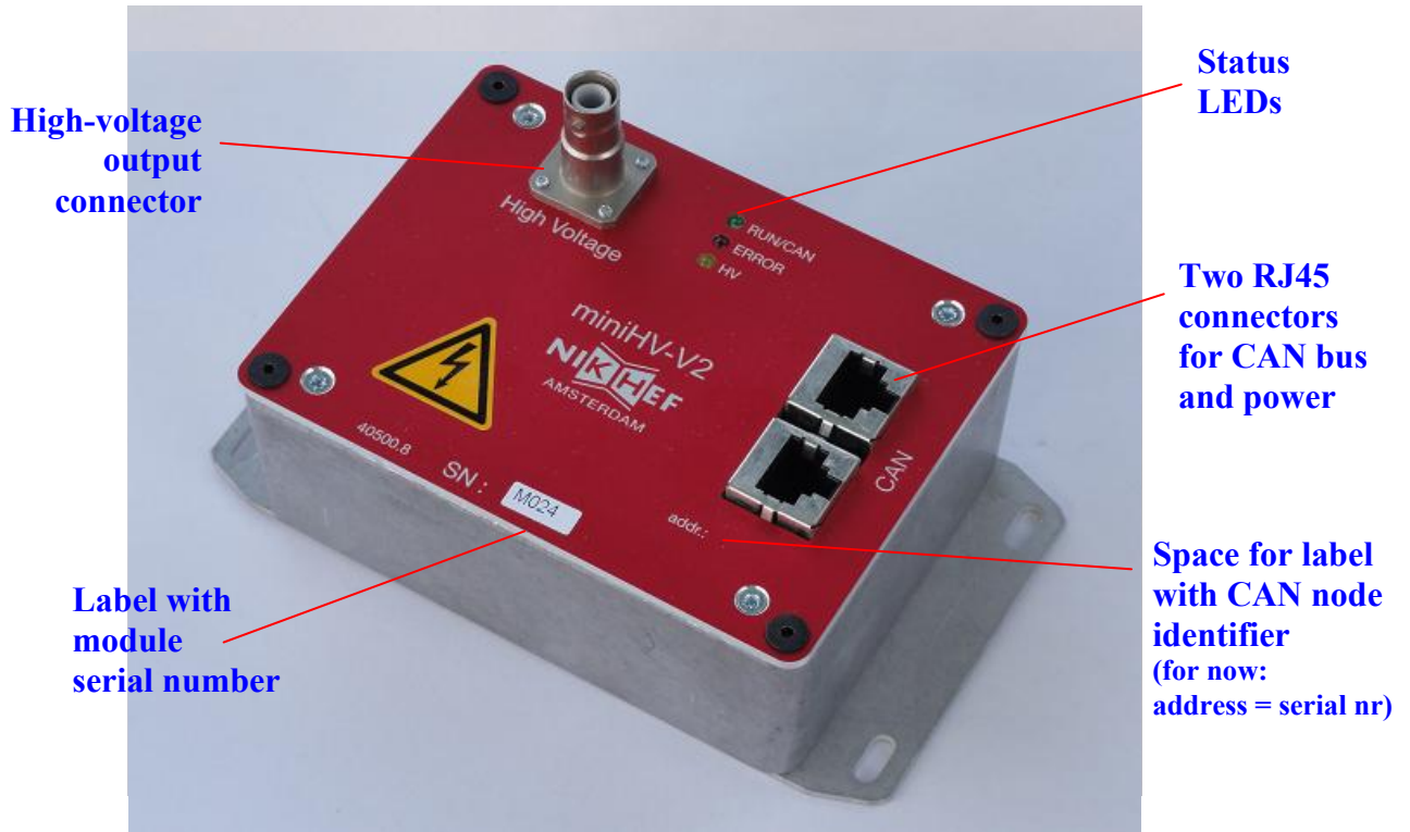
Figure 1. The miniHV high-voltage powersupply module. The RJ45 plugs carry the CAN-bus lines and power for the module and high-voltage generation. The module has two of these connectors for daisy-chaining multiple miniHV modules.
