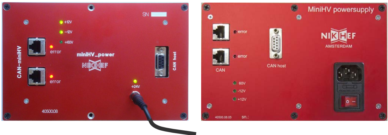
Figure 4. Left picture: miniHV powersupply unit frontpanel, showing incomplete and/or unterminated CAN bus branches indicated by the red ‘error’ LEDs being on, and the 60V supply which is off due to this, indicated by the green ‘+60V’ LED being off. Right picture: frontpanel of the new miniHV powersupply unit, featuring a direct connection to a net power outlet.
