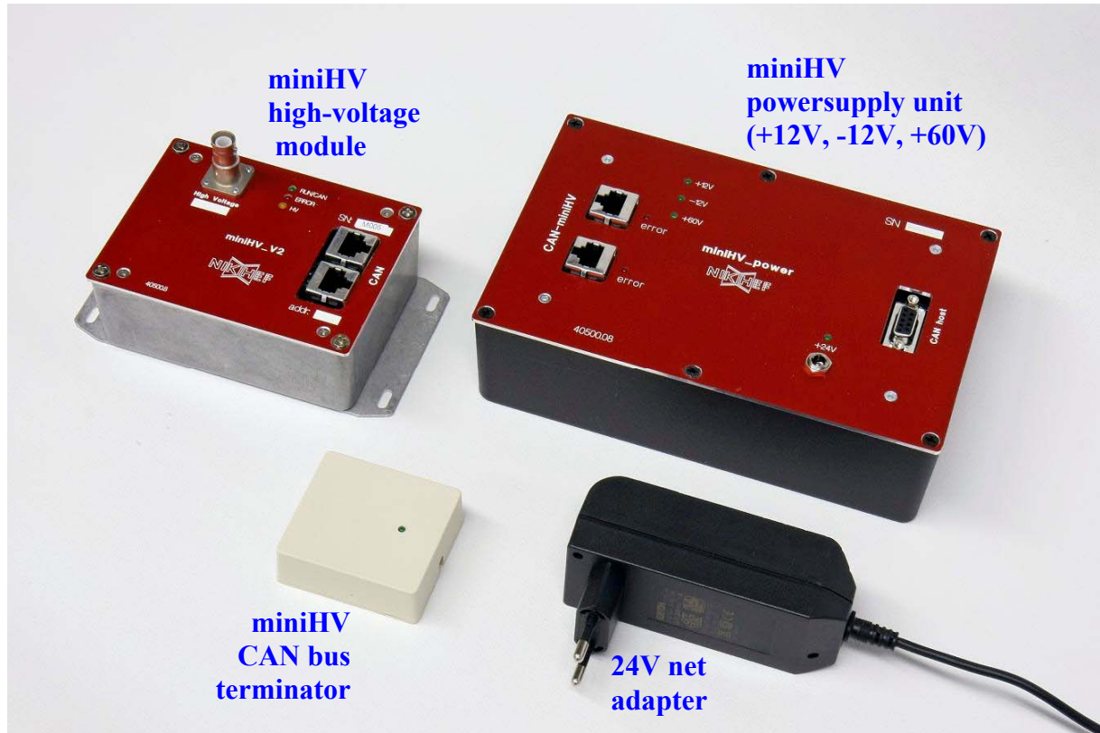
Figure 2. The miniHV system components. NB: the powersupply unit has been redesigned to connect directly to a power outlet and to not require a 24V net adapter (see Figure 4, picture on right), for reasons of improved grounding.
