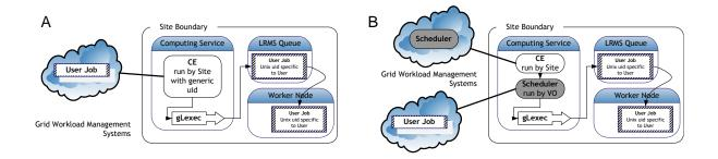
**Figure 1.** Flow of a grid job through the Grid Computing Service and the LRMS for the Site-CE scenario (A) and the VO-CE scenario (B). White boxes represent processes run under control of the site, gray boxes are processes run by a (generic) VO uid on the Grid Computing Service system, and dashed boxes represent processes or Jobs run or held with a Unix uid associated uniquely to the User owning the workload of this Job.
