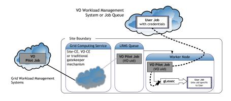
Figure 2. Flow of a grid job through the Grid Computing Service and the LRMS for the pilot job scenario. The Pilot Job can be submitted to the LRMS in various ways that are not relevant to the scenario. Shading as in Fig. 1.
