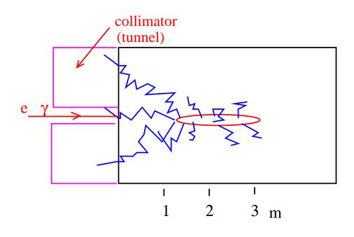
Unfortunately the diameter of the hole should be large enough. The angular spread of initial electron beams and Compton photons is very narrow,  $\sigma_{\theta} \sim 0.1$  mrad. However, due to beam repulsion the angular spread is up to 10 mrad for all disrupted particles and about 2 mrad for electrons with full energy at E = 100 GeV (20 cm at the distance 100 m). So, the diameter of the tunnel should be about 1 m; (checked: helps)
