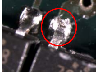
IC588 pin 5 open; repaired (~23-jul-2007)
