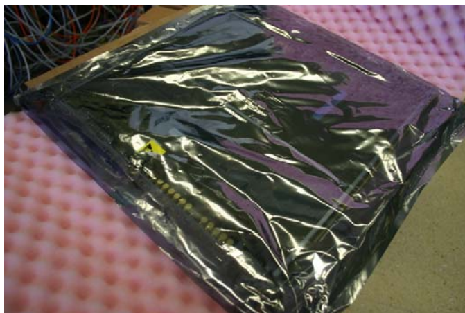
Figure 6: Use an anti-static bag to package the modules into the special boxes.
