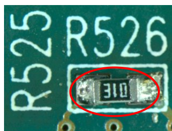
Figure 8: R526 should be 0Ω (not 1M)
