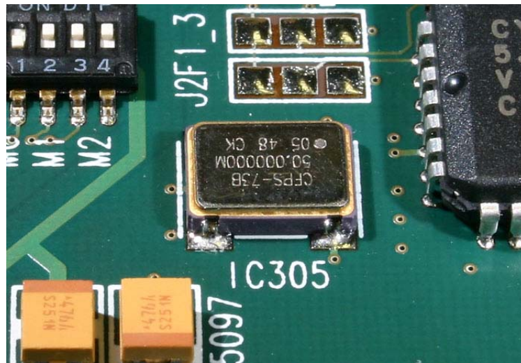
Figure 18: IC305 has wrong orientation
