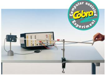
Measurement of sound velocity through a metal rod (CBT 3.22)
