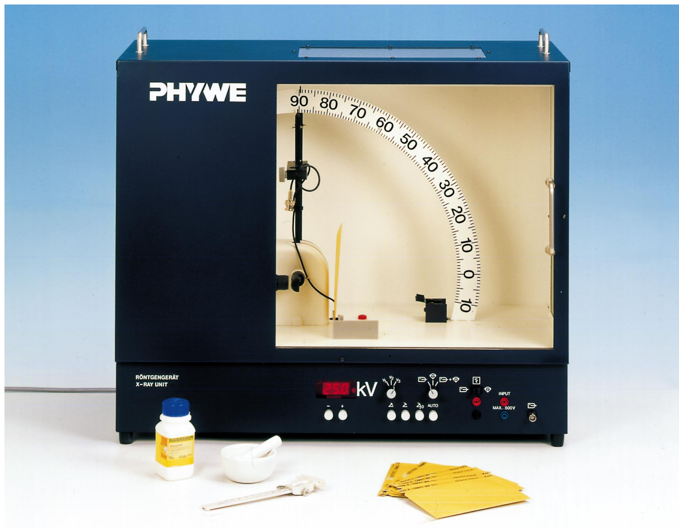
Fig. 1: Experimental set-up for Debye-Scherrer photographs.
