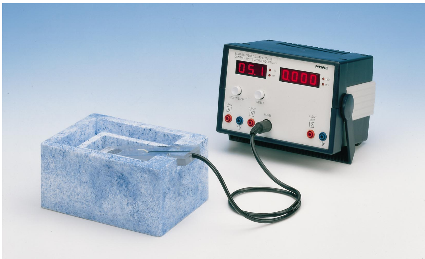
Fig. 1: Experimental set-up for determining the transition temperature of a HTSC.
