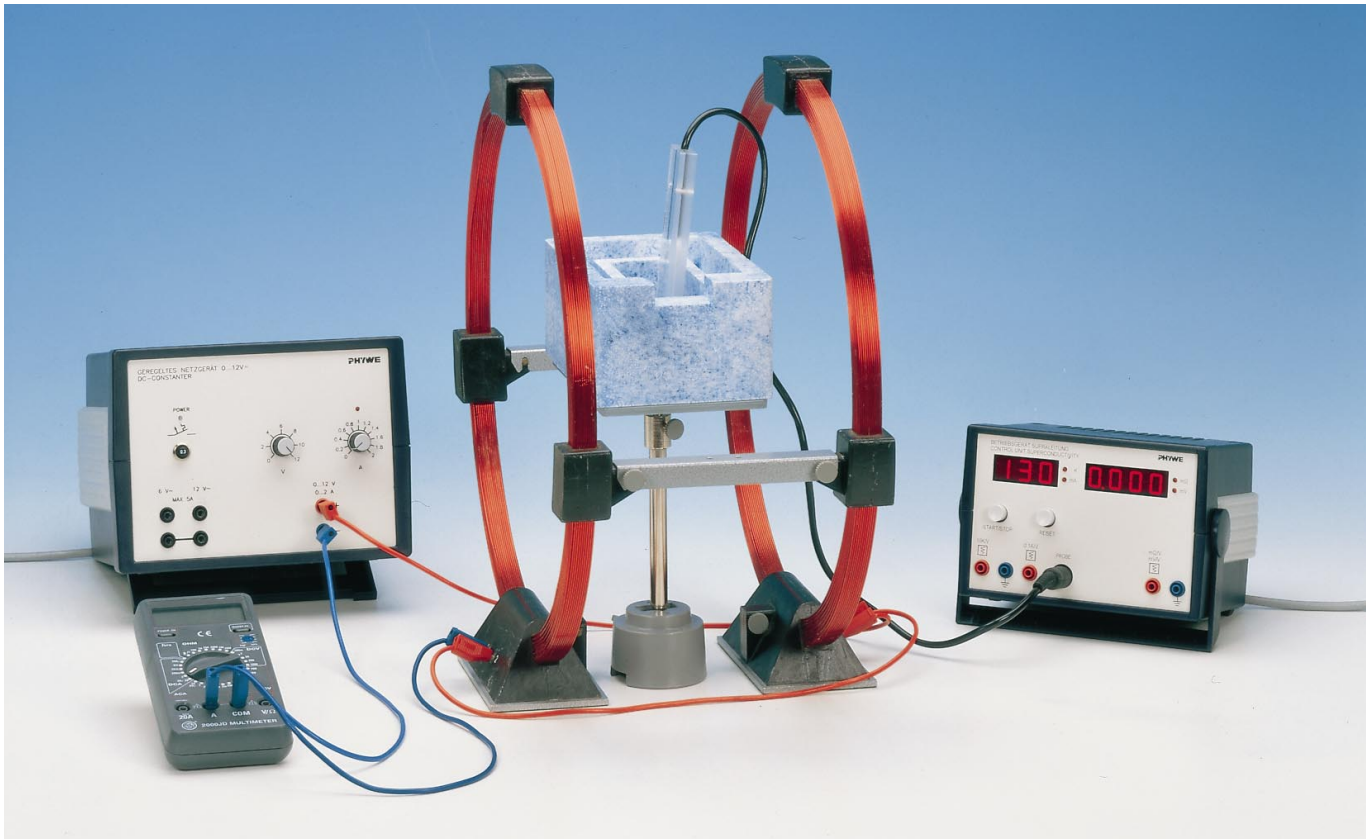
Fig. 2: Experimental set-up: Influence of current and B-field.
