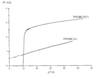
ure resistance as a function of the difference of temperature. Temperature must increase very slowly in order to obtain a reliable value of the critical temperature. Stop measurement once the difference of temperatures increases above 50 K. Plot the R(T) graph of the superconductor.
