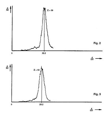
Figs. 2 to 6 show on an number of measurement examples the spectra of X-ray-fluorescence radiation obtained with barium, iodine, indium (if available), cadmium and strontium. Fig. 7 shows the calibration lines of <sup>137</sup>CS and <sup>241</sup>Am plotted on the same energy scale.
