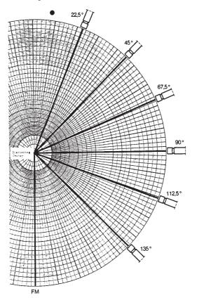
Fig. 3: Arrangement of the extra lead brick for shielding direct radiation (P = source, S = Scattering medium, D = detector).  $\land$  P
