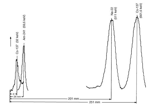
Fig. 5: Energy of known peaks as a function of the position of the xyt recorder.
