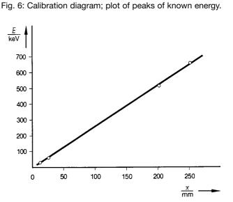
1. The set-up is calibrated by recording peaks of known energy: Cs-137, Am-241 and Na-22. Plot the energies on a graph as a function of the position of the xyt recorder (x).
