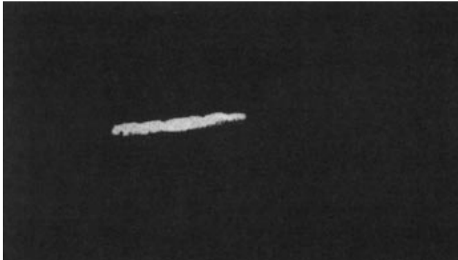
Fig. 6: Track generated by an \alpha -particle.
