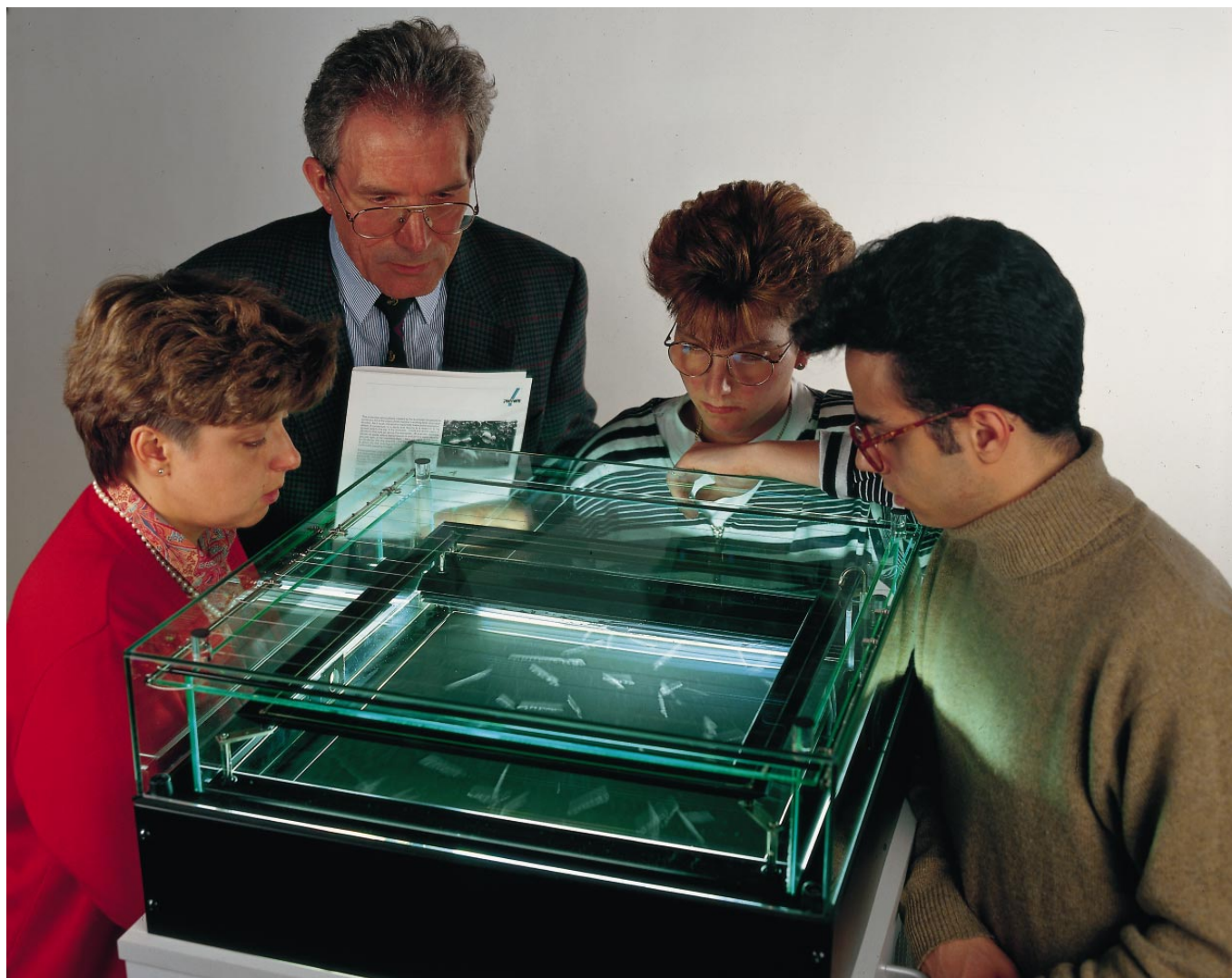
Fig. 1: Experimental set-up: Diffusion cloud chamber.
