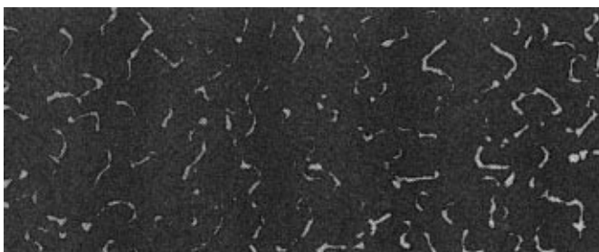
Fig. 11: Track generated by protons-electrons and Compton-electrons.
