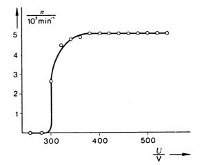
Fig. 5: Counting rate at constant activity, as a function of the counter tube voltage.
