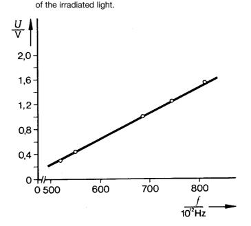
Fig. 2: Voltage of the photo-cell as a function of the frequency
