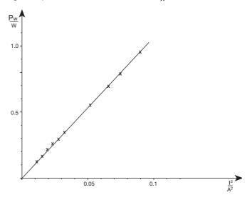
also causes a large change of  $\tan\varphi$  and  $\cos\varphi$  (and thus a change of real power  $P_W$ ). This explains why the measurement points deviate from the straight lines in figs. 6 and 7.
