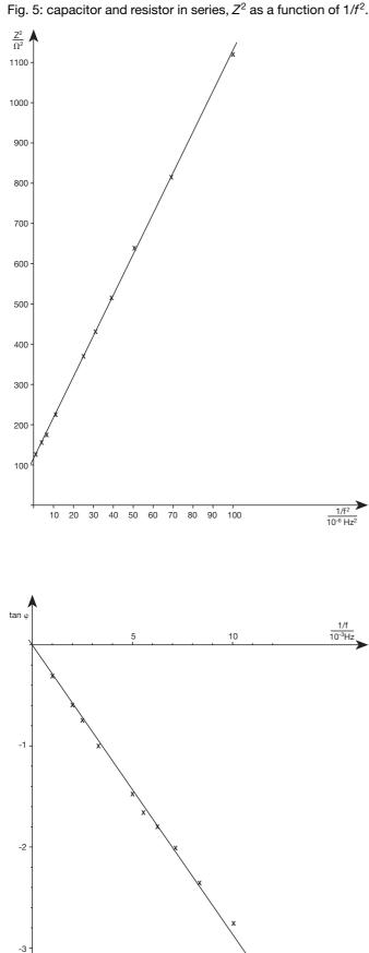
or in series,  $Z^2$  as a function of  $1/f^2$ . Fig. 7: capacitor and resistor in series,  $P_W$  as a function of  $I^2$ .
