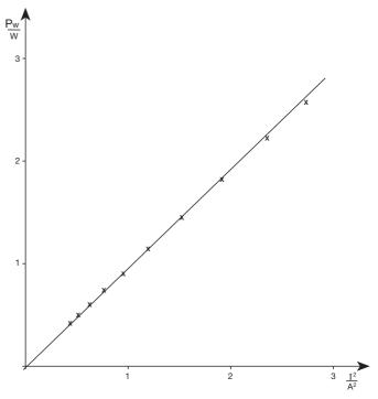
Fig. 4: self-inductance and resistor in series,  $P_W$  as a function of  $I^2$ .
