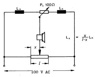
Fig. 3: Circuit for measuring inductances.
