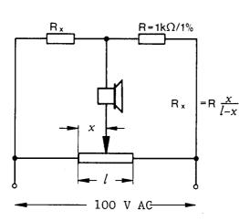
Fig. 2: Circuit for measuring resistance.
