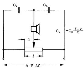
Fig. 4: Circuit for measuring capacitances.
