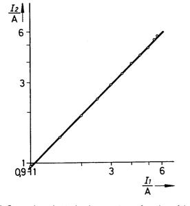
Fig. 5: Secondary short-circuit current as a function of the primary current in the transformer.
