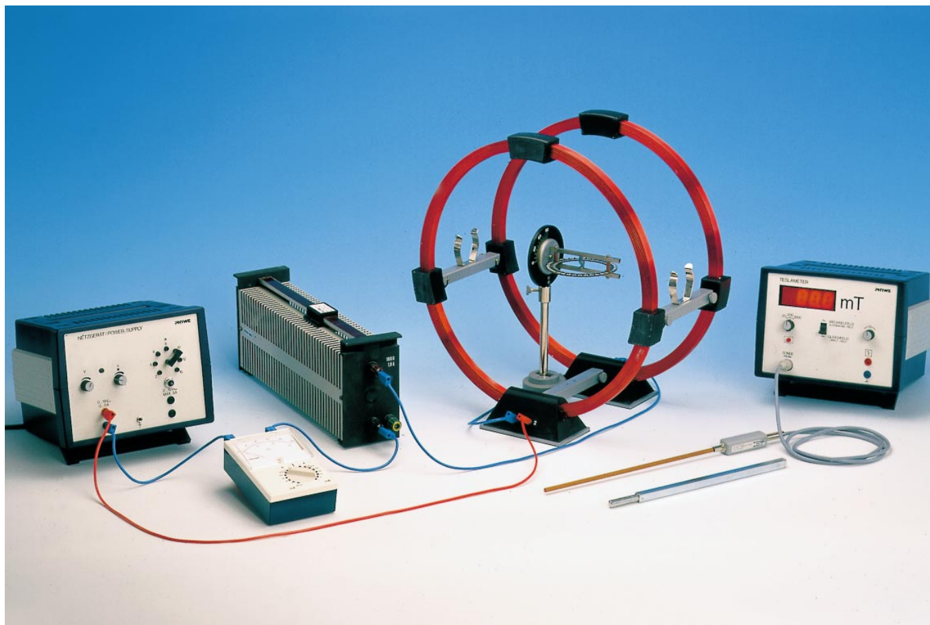
Fig. 1: Experimental set-up to determine the earth's magnetic field.
