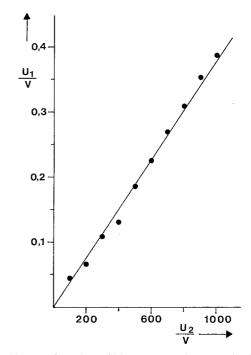
Fig. 5: U<sub>1</sub> as a function of U<sub>2</sub> measured on a spherical capa-
