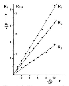
Fig. 4: U<sub>1</sub> as a function of U<sub>2</sub> measured on conducting spheres with three different diameters.
