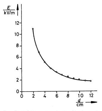
Fig. 4: Electric field strength as a function of the plate spacing.
