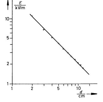
With constant voltage U, the field strength E varies in inverse proportion to the spacing d.
