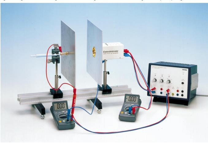
Fig. 1: Arrangement for measuring the electric field strength as a function of the voltage and the plate spacing.
