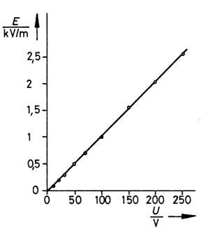
Fig. 3: Electric field strength as a function of the plate voltage.
