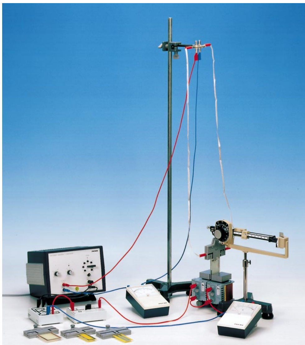
Fig. 1: Experimental set-up: Current balance. Force acting on a current-carrying conductor.
