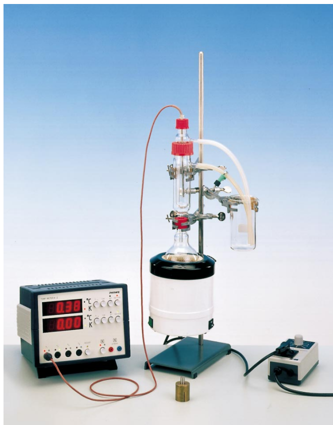
Fig. 1: Experimental set-up: Boiling point elevation.
