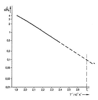
Fig. 3: Natural logarithm of vapour pressure p as a function of the reciprocal of the temperature (117):  $T_b = \text{boiling point at normal pressure.}$
