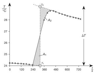
Fig. 3: Temperature-time diagram for a measurement example.
