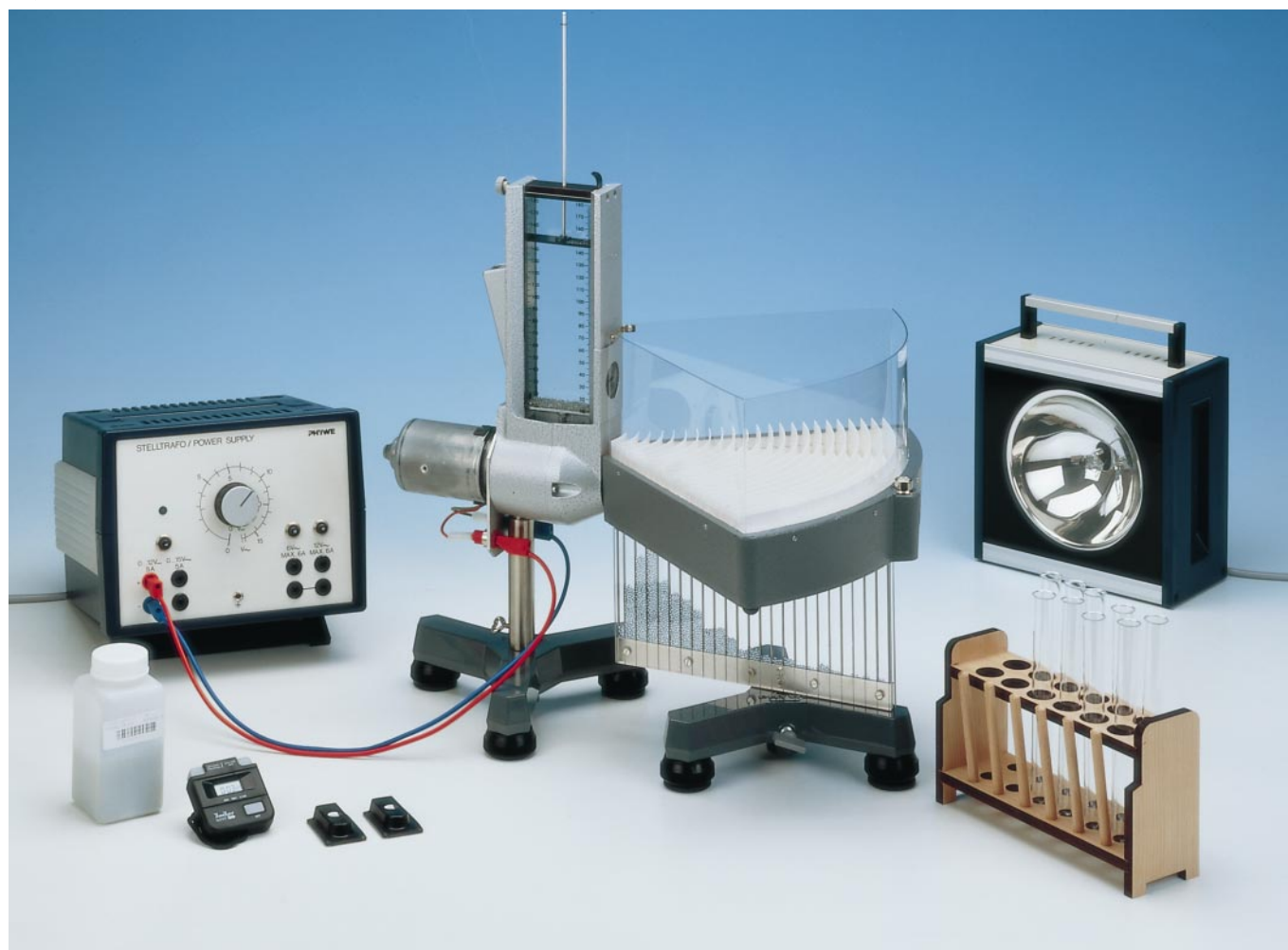
Fig. 1: Experimental set-up: Maxwellian velocity distribution.
