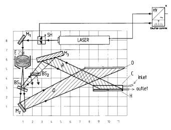
Experimental set-up for real-time procedures as a holographic interferometer for a bending plate (\* only required for 5 mW laser)
