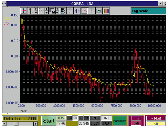
Fig. 8: Measurement of the signal spectrum with a signal peak 9525 Hz for 38 averagings. The real measurement has a signal peak at 9052 Hz.
