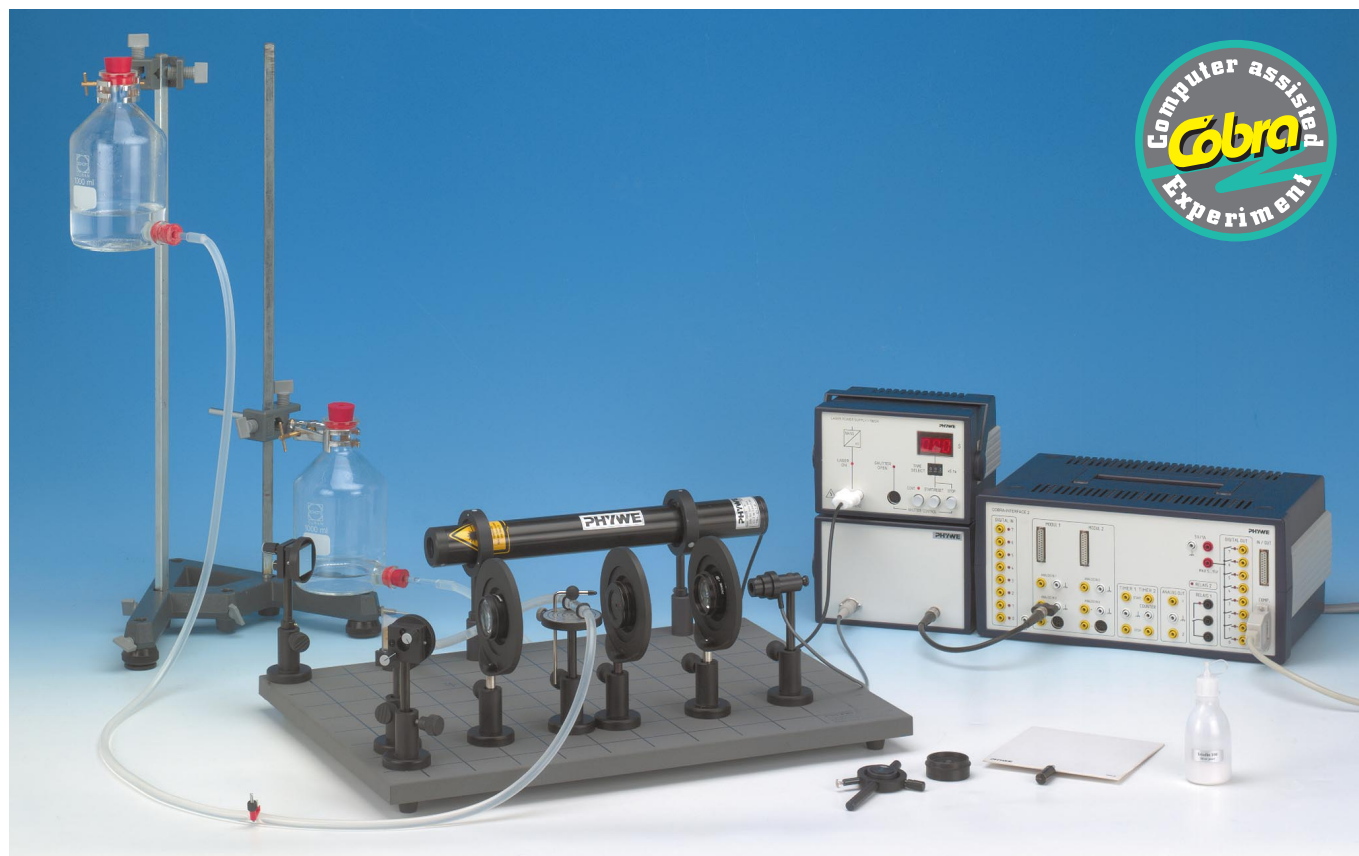
Fig.1: Complete set-up of the experiment: LDA – Laser-Doppler-Anemometry.
