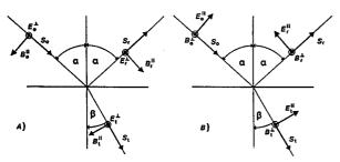
In Fig. 3 A) the electric vector  $E_0^+$  of the incident light wave oscillated perpendicular to the plane of incidence; the magnetic vector  $B_0^+$  oscillates parallel to this according to (2). According to the law of the continuity of tangential components (components that oscillate parallel to the surface of the object) and taking the direction of the beam into account, the following applies:
