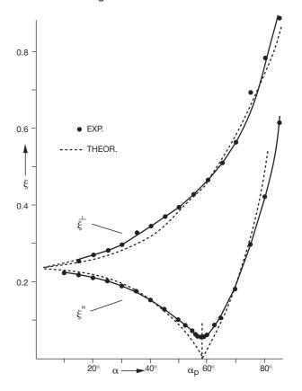
If after reflection the electric vector oscillates at the azimuth angle  $\omega$ , then a rotation of the plane of polarization through the angle  $\psi = \delta - \omega$  is produced. For the comonents parallel and normal to the plane of incidence:
