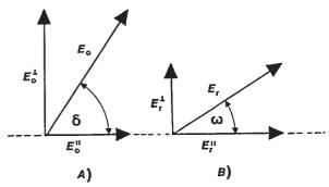
Fig. 6: Rotation of the direction of oscillation by reflection.
