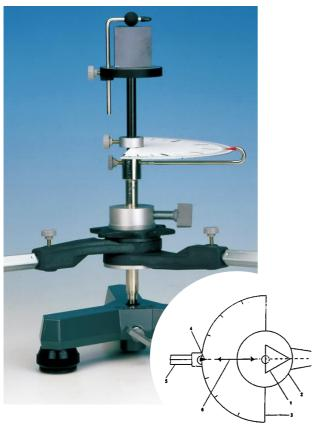
Fig. 2: Articulated radial holder with prism arrangement for finding the reflection at  $\alpha=0^{\circ}$
