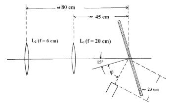
Due to its rough surface, the zinc-sulphide screen provides a practically ideal diffuse reflecting Lambert source.
