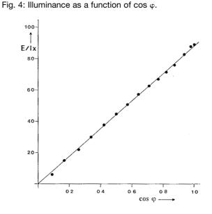
According to (1), the luminous flux is proportional to  $\cos \phi$  within a spatial angle (Lambert's law). According to (3), this also is valid for the illuminance, which can be determined by means of a luxmeter.
