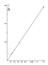
Fig. 4: Focal length of first and higher order of the zone plate as a function of the reciprocal value of the order.
