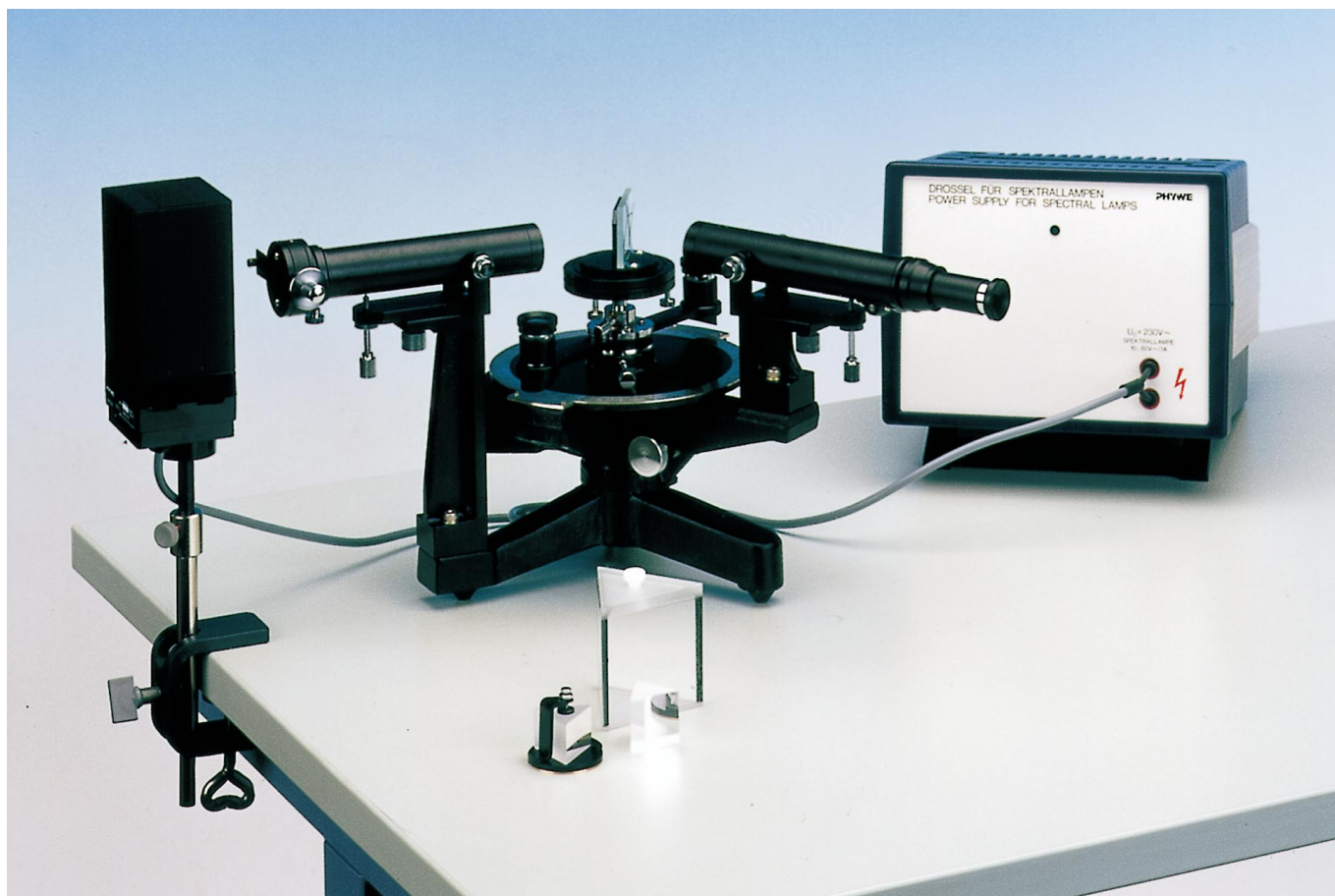
Fig. 1: Experimental set-up for determining dispersion in liquids.
