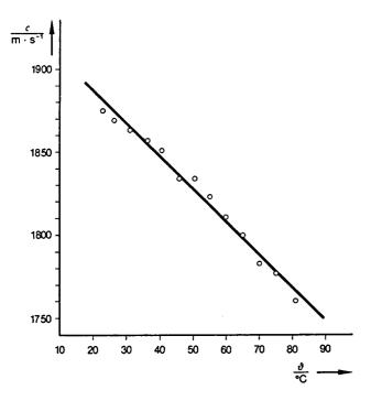
Velocities of sound with temperature coefficient
