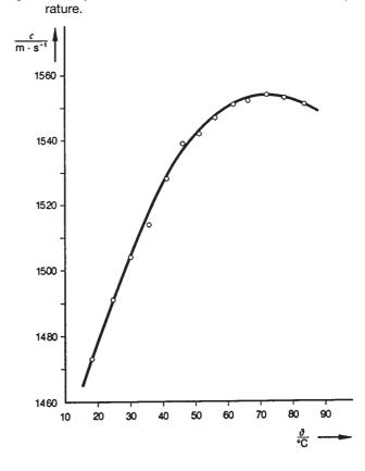
Fig. 2: Velocity of sound in water as a function of the tempe-
