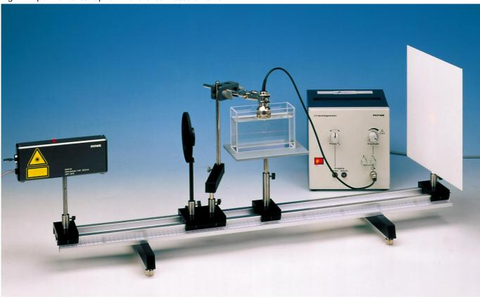
Fig. 1: Experimental set-up for interference measurements.
