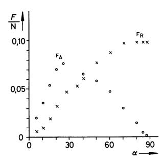
Fig. 4: Lift  $F_A$  and resistance  $F_R$  of a flat plate as a function of the angle of incidence.
