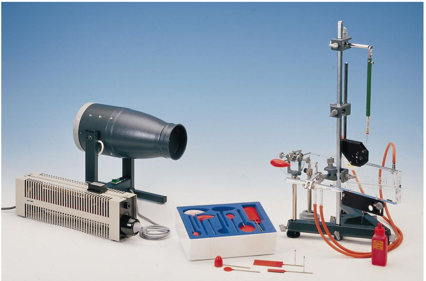
Fig. 1: Experimental set up for determining the resistance to flow.
