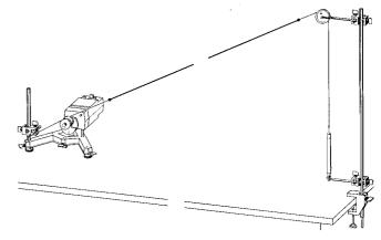
In the first section of the experiment, the dependency of the wave length  $\lambda$  on the excitation frequency *f* with constant tensile stress on the quadrangular rubber strip is determined. The frequencies of the rubber strip, varying with the electric motor (regulated operating mode) are calculated with the help of a stroboscope. It is suggested to work in a darkened room, with a bright background. The wave length is determined by doubling the distance between two wave knots.
