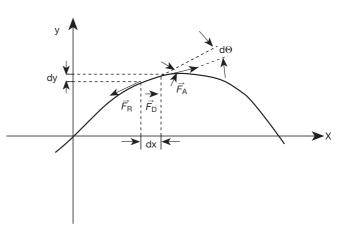
Fig. 4: The relationship of force in a rope wave.
