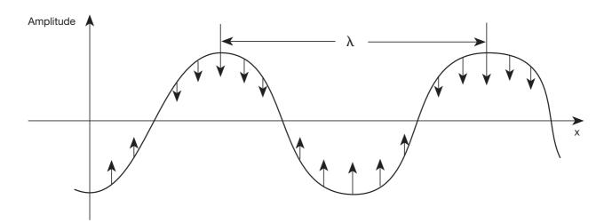
Fig. 2: To define the wave length of a harmonic wave.
