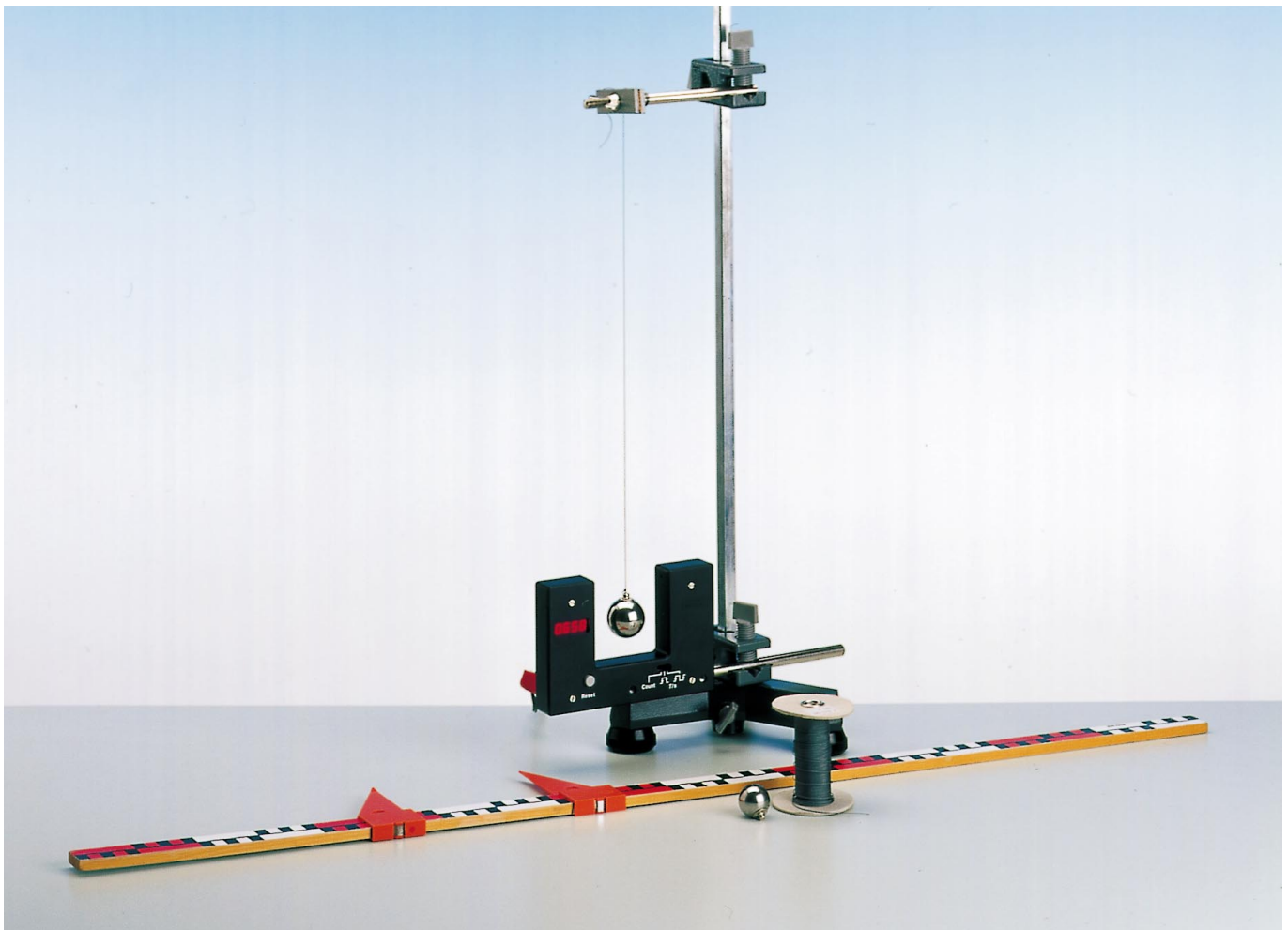
Fig. 1: Experimental set up for determining the oscillation period of a mathematical pendulum.
