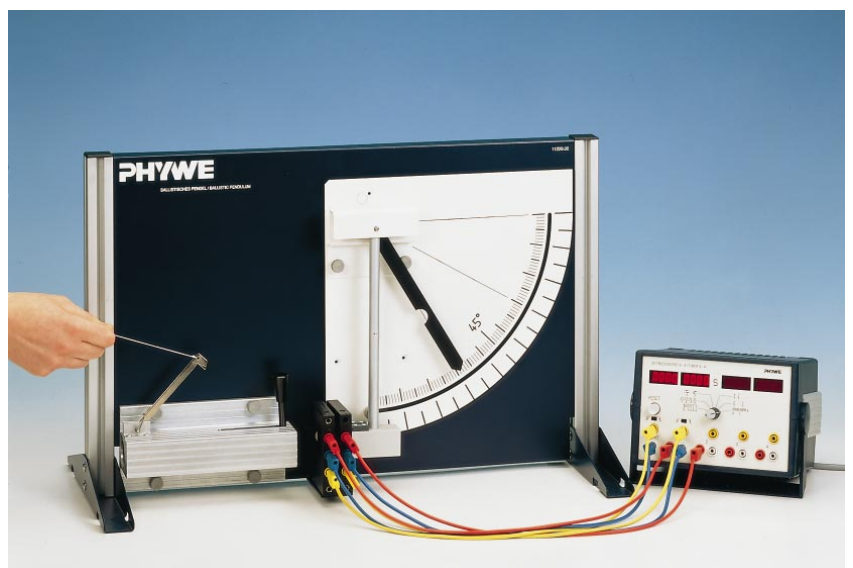
Fig. 4: Experimental set-up with supplement for direct measurement of the initial velocity of the ball.
