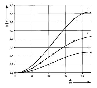
Fig. 4: Maximum height of projection h as a function of the angle of inclination  $\phi$  for the initial velocities as in Fig. 1:
