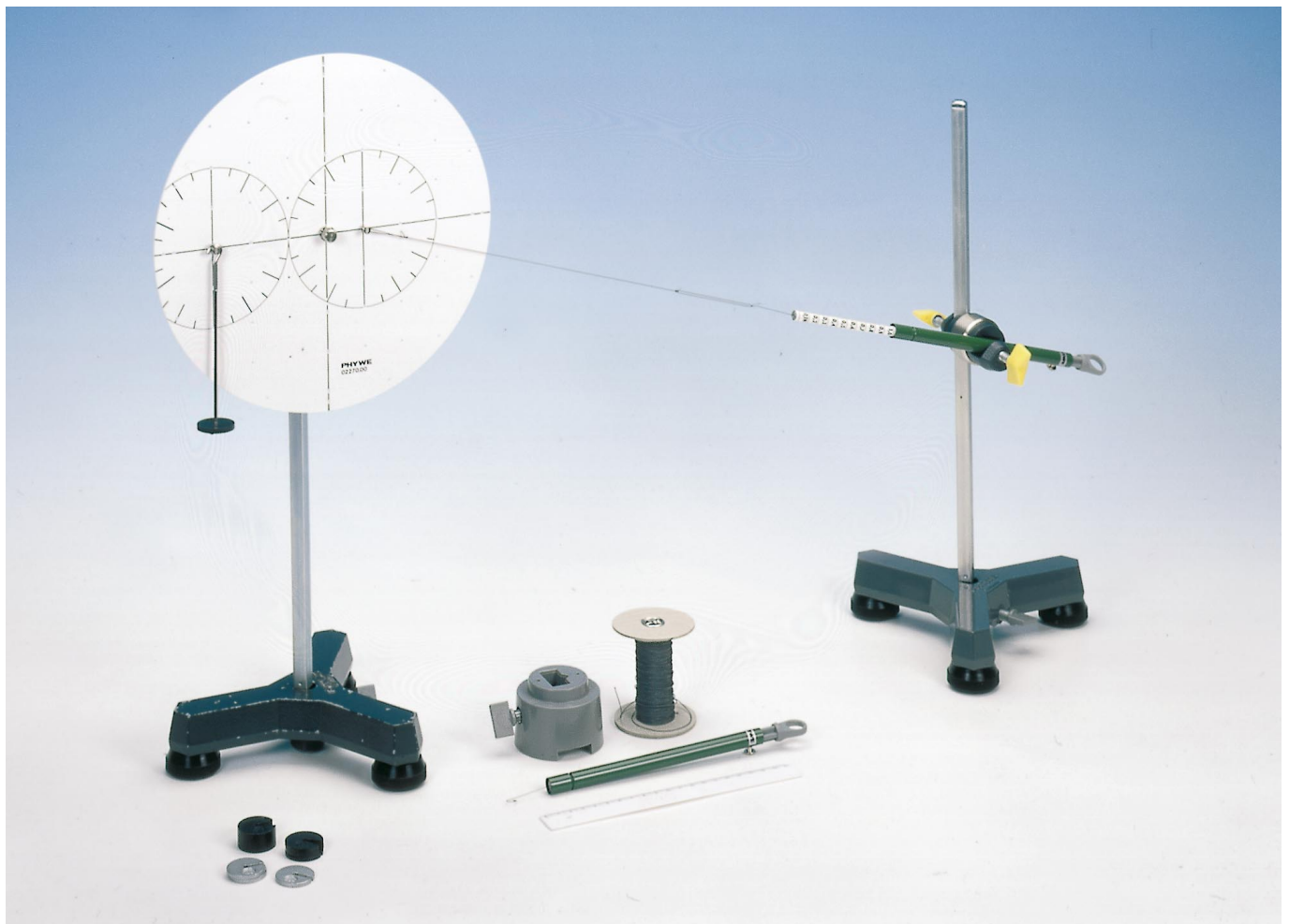
Fig.1: Experimental set-up for investigating moments in equilibrium.
