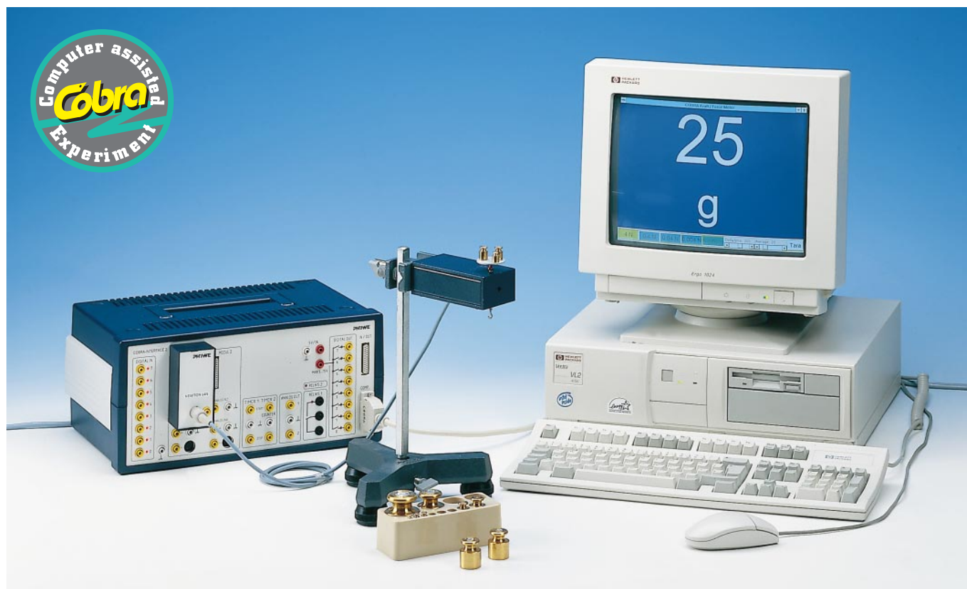
Fig.1: Experimental set-up: Force measurement with PC interface.
